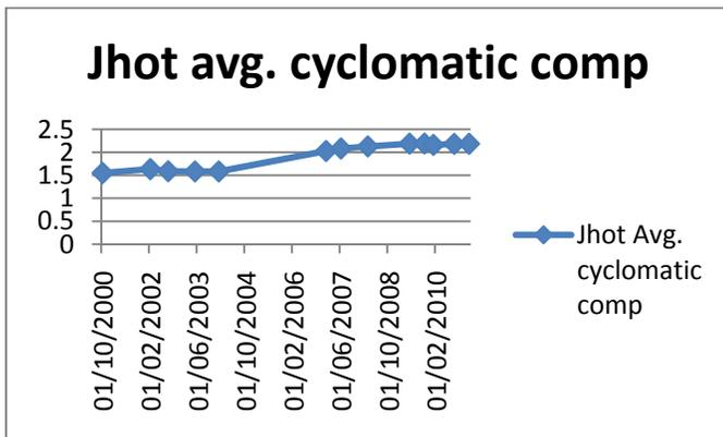
Figure 21. Graph showing average cyclomatic complexity for different releases of JhotDraw.
